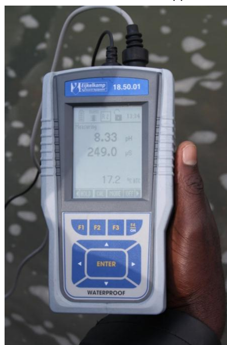
Figure 4-2 : Measuring of pH, temperature and conductivity in the Buzi River Basin, Zimbabwe June 2010.
