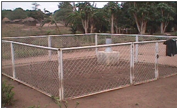
Rainfall gauges are important to monitor the available water resources and possible changes in the climate
