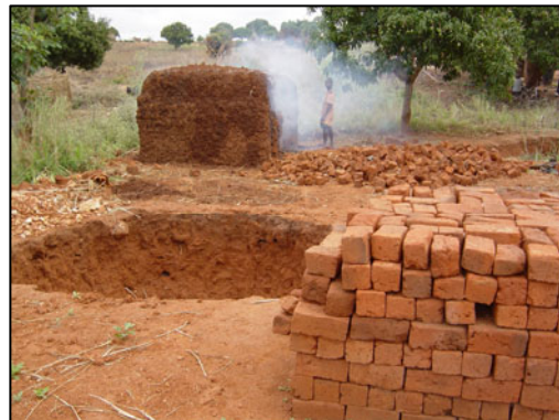
The typical red clayey soil of the western part of the river basin may be used to make bricks
