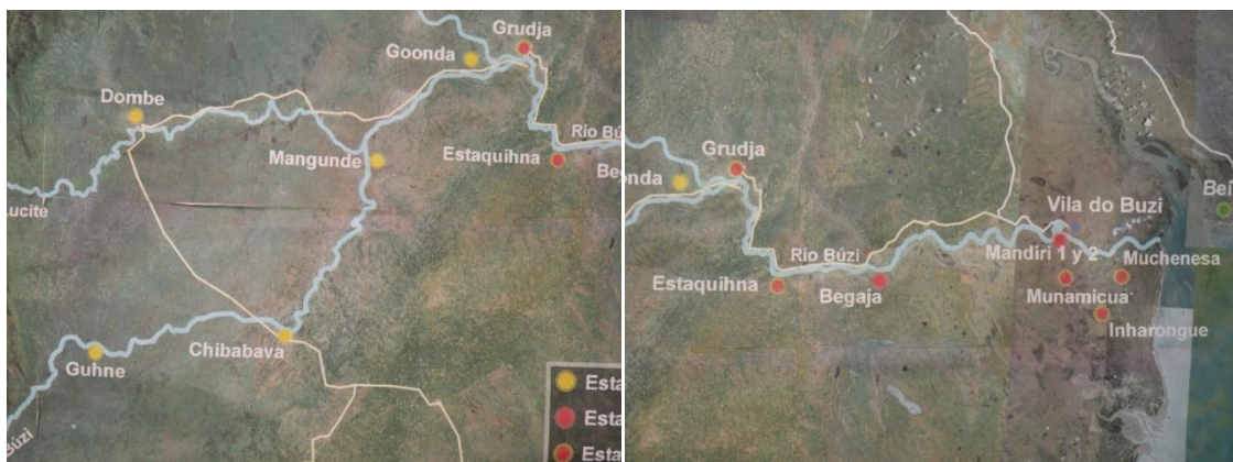
Figure 7-6: Buzi Flood Warning System. The yellow dots are the upstream monitoring stations and the red dots are the response centres in flood-prone areas.
