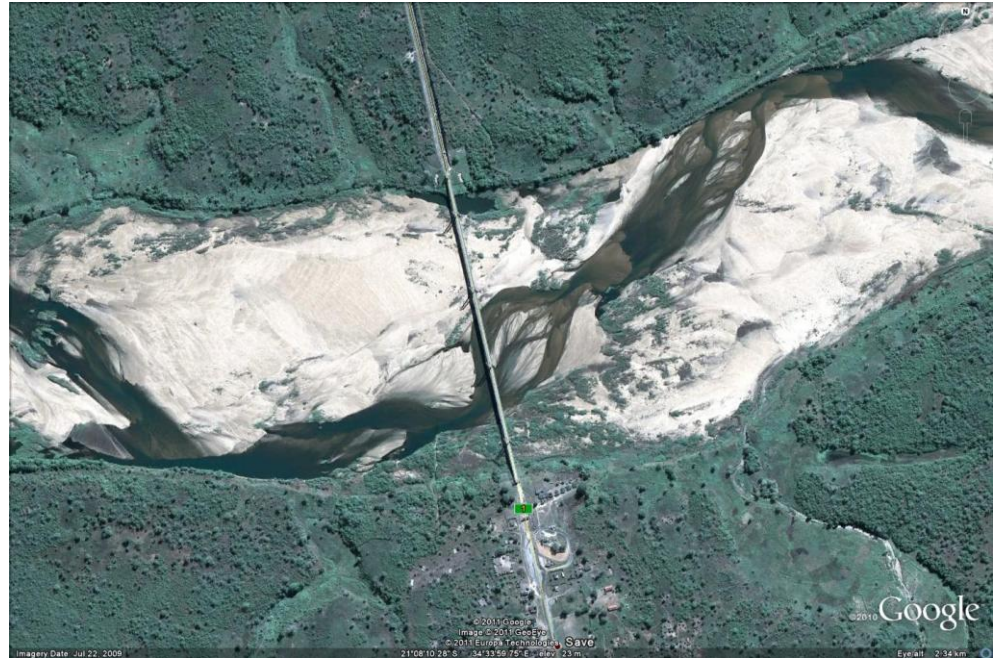
Figure 16 Villa Franca do Save. The national highway EN1 crosses here (the only road crossing in Mozambique). A key hydrometric station is located here. The stretch is typical for Save River in Mozambique. (Source: Google Earth)
